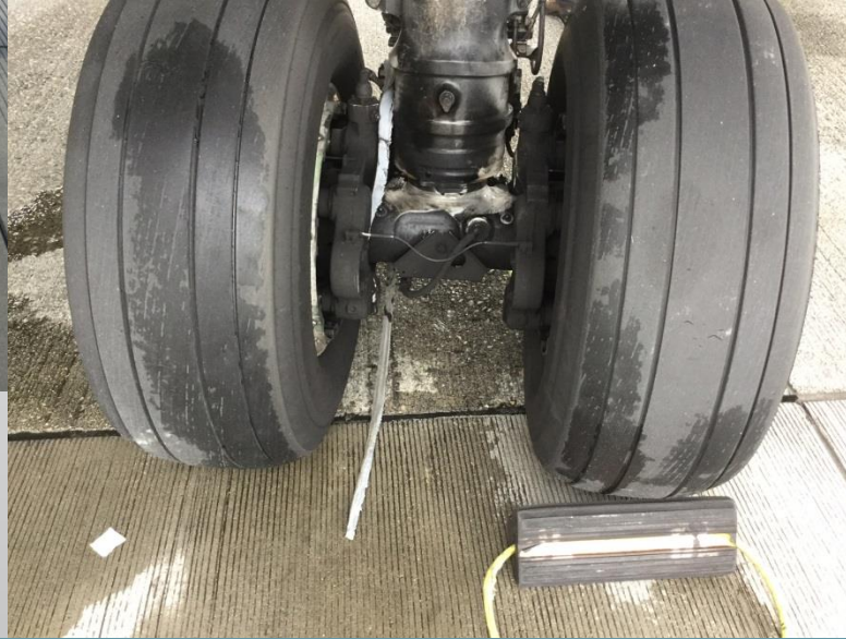
Failed Joint Seal at Runway 16L/34R
